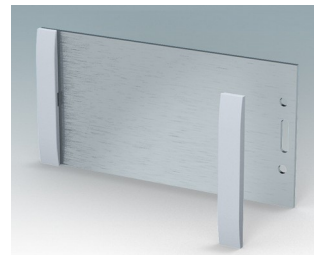
M5100520 Front/rear panel kit AN (size 2 & 4) Aluminium Matt anodised 129.5x2x65.1mm
